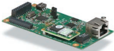
Wireless Ethernet Internal Card 802.11 b/g Wireless
