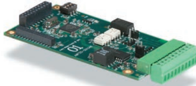
Current Loop Card Current Loop/RS485/RS422.
