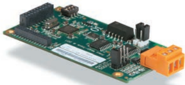
Analogue Output Card 0-10 VDC and 4-20 mA.
