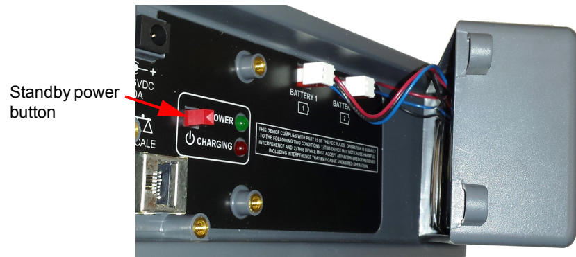
Figure 2.6 Battery pack connections
