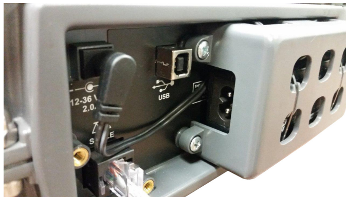
Figure 2.4 AC power block
