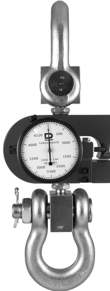
Figure 2.3 Tensile model with adapters and shackles
