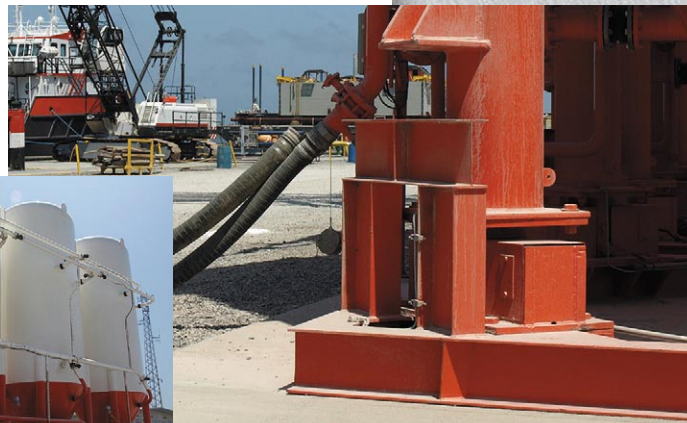
M-I SWACO weighs tanks filled with imperative substances for the drilling industry using Avery Weigh-Tronix Weigh Bars and Model 1310 indicators. The tanks can weigh up to a million pounds each.
