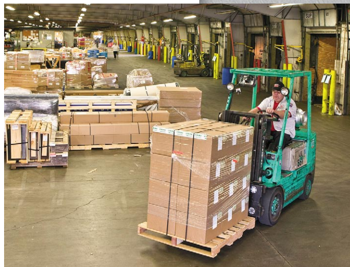
Lakeville Motor Express weighs and bills freight using the FLSC forklift scale. Its scale carriage contains two metal plates paired with Weigh Bar weight sensors.
